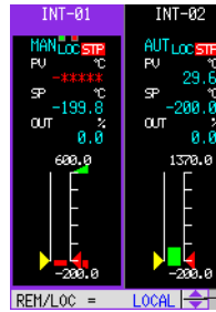
Window for switching between remote and local
